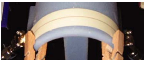
Figure 1. Photograph of the fabricated microstrip trace curved over a surface.
