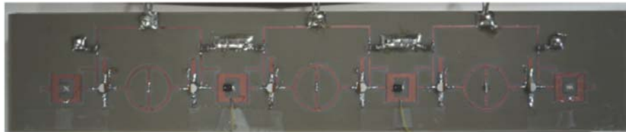
Figure 8. Fabricated push-push oscillator array.
