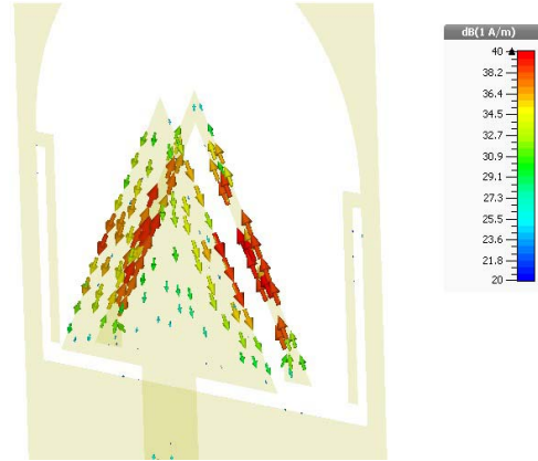
Figure 5. The current distribution of the proposed antenna at f = 7.5 GHz, H = 1.5 mm, and V = 7.3 mm.
