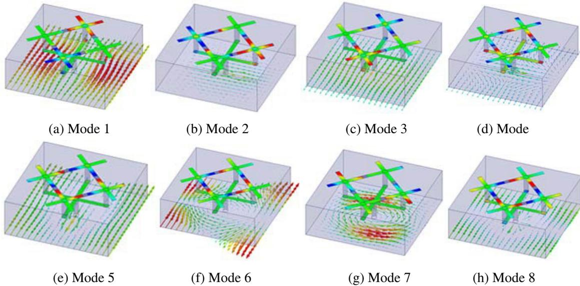
**Figure 4.** Simulated distribution of the electric field  $z$  component on the metallic cross and surface current on the ground plane for different eigenmodes.
