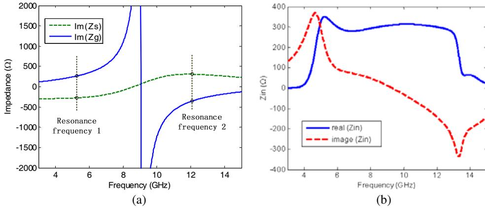
**Figure 5.** Calculated effective surface impedance of (a)  $Z_s$ ,  $Z_g$  and (b)  $Z_{in}$ .
