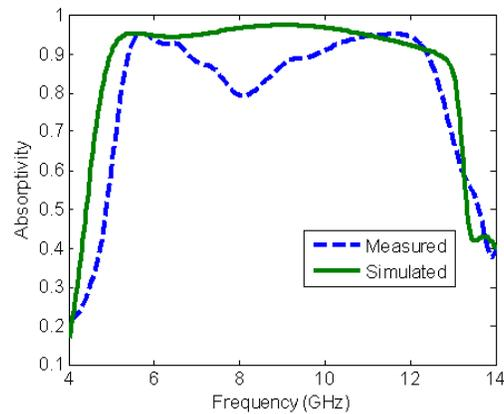
**Figure 7.** Simulated and measured absorptivity of the  $19 \times 19$  absorber array.
