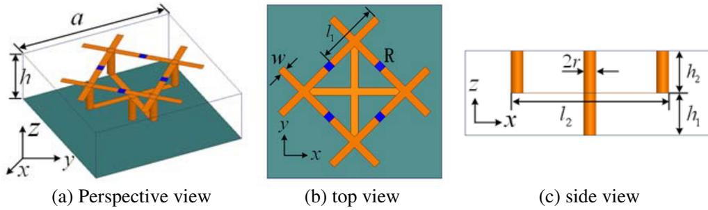
**Figure 1.** Geometry of the proposed absorber unit cell with structure parameters are  $a = 12$ ,  $h = 4h_1 = h_2 = 2$ ,  $w = 0.5$ ,  $l_1 = 4.4$ ,  $l_2 = 7r = 0.3$  (unit: mm).
