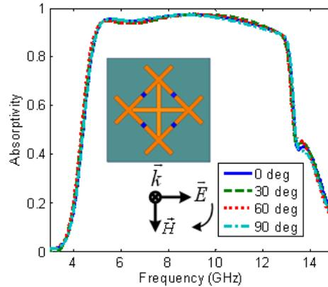
**Figure 2.** Simulated absorption for different polarization angles for the normal incidence.
