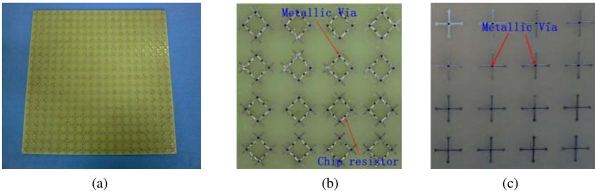
**Figure 6.** (a) Photo of the fabricated  $19 \times 19$  fractal tree absorber and (b) zoom in the top layer and (c) middle layer.
