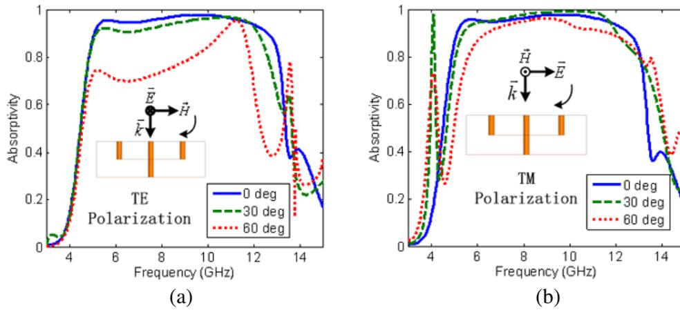
**Figure 3.** Simulated absorption for different oblique incidence angles, (a) for TE polarization, (b) for TM polarization.
