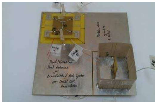
Figure 6. The prototype antenna fabricated with control circuits.
