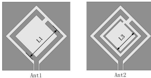
**Figure 2.** Two improved prototypes of the proposed antenna.
