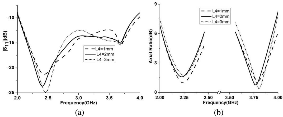
**Figure 10.** Simulated  $|S_{11}|$  and AR with different  $L_4$ 's for the proposed dual-band dual-sense antenna. (a)  $|S_{11}|$ , (b) AR.
