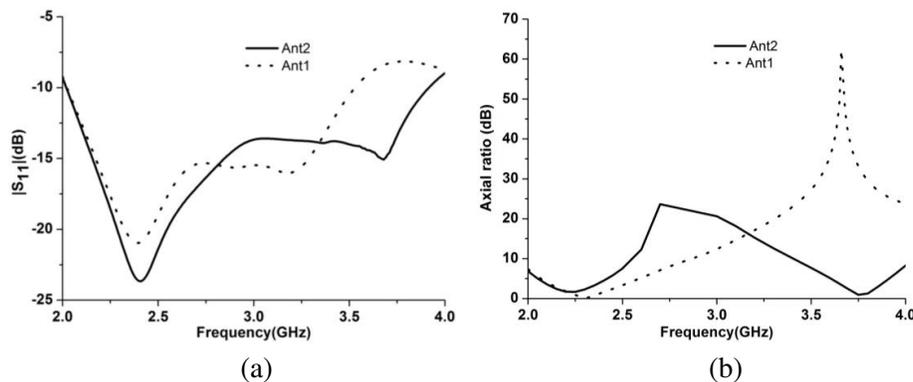
**Figure 3.** Simulated  $|S_{11}|$  and AR for Ant 1 and Ant 2, (a)  $|S_{11}|$ , (b) AR.
