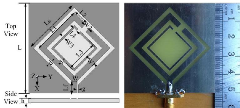
**Figure 1.** Geometry of the proposed antenna.
