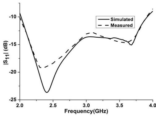
Figure 5.  $|S_{11}|$  of the proposed dual-band dual-sense CP antenna.
