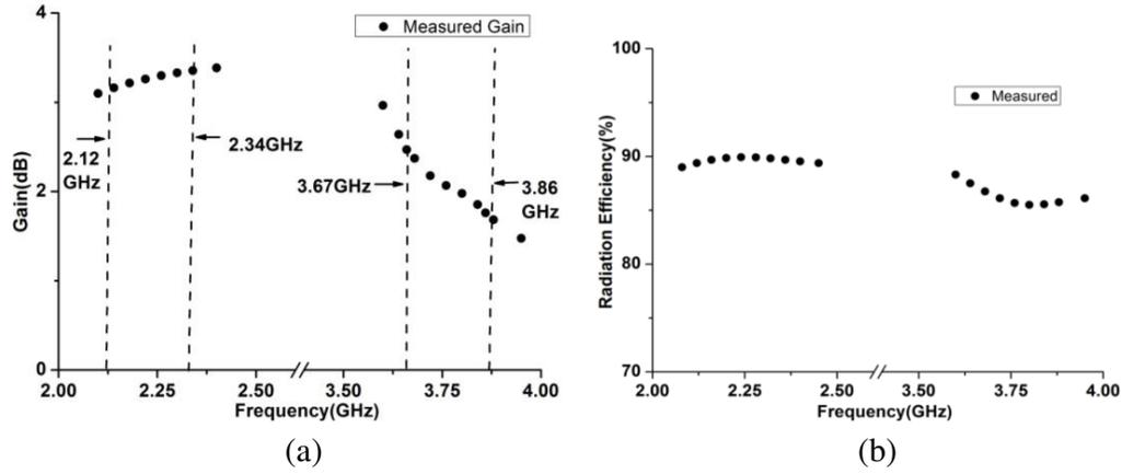
**Figure 8.** Measured peak gain and radiation efficiency of the proposed antenna: (a) Gain, (b) radiation efficiency.
