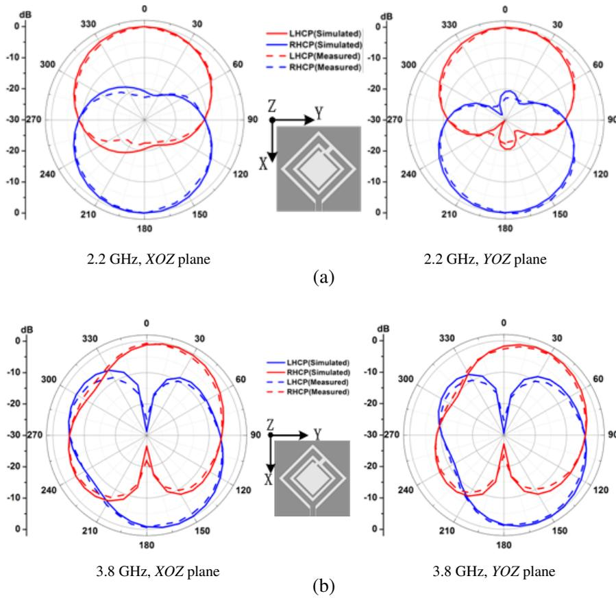
Figure 7. LHCP/RHCP radiation patterns of the proposed antenna in  $XOZ$  and  $YOZ$  planes. (a) 2.2 GHz, (b) 3.8 GHz.
