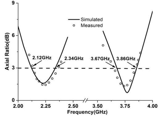
Figure 6. AR of the proposed dual-band dual-sense CP antenna.
