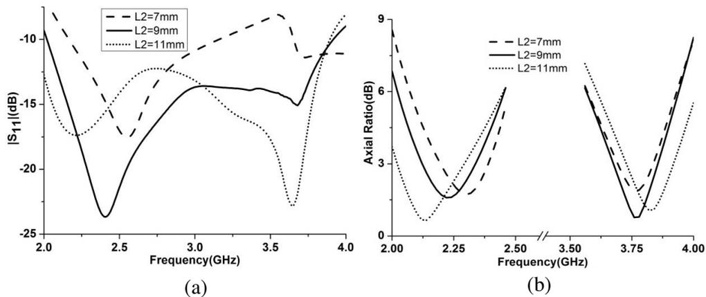
**Figure 9.** Simulated  $|S_{11}|$  and AR with different  $L_2$ 's for the proposed dual-band dual-sense antenna. (a)  $|S_{11}|$ , (b) AR.
