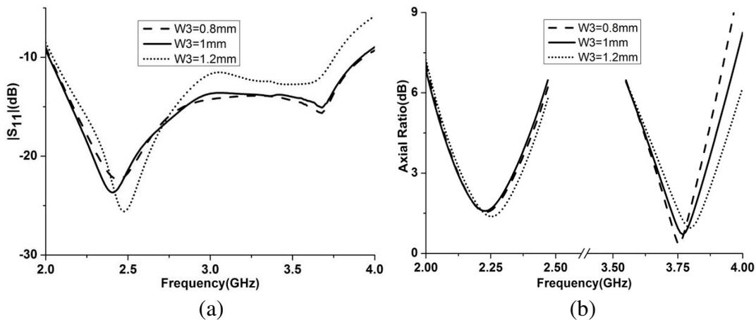
**Figure 11.** Simulated  $|S_{11}|$  and AR with different  $W_3$ 's for the proposed dual-band dual-sense antenna. (a)  $|S_{11}|$ , (b) AR.
