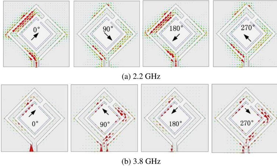
**Figure 4.** Surface current distributions of the proposed antenna 2 in  $0^\circ$ ,  $90^\circ$ ,  $180^\circ$  and  $270^\circ$  phase. (a) 2.2 GHz. (b) 3.8 GHz.
