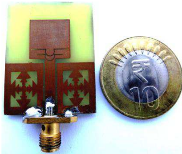
Figure 9. Fabricated prototype of antenna.
