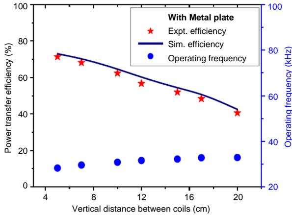
**Figure 6.** Both the simulated and experimental resonant frequency characteristics of optimum energy transfer efficiency of the wireless energy transfer system with metal plate.
