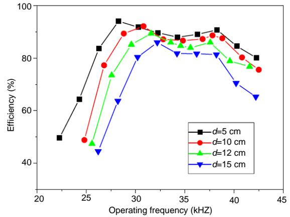
**Figure 4.** Measured frequency characteristics of energy transfer efficiency for different vertical spacing between the transmitting and receiving resonant coils of wireless energy transfer system.
