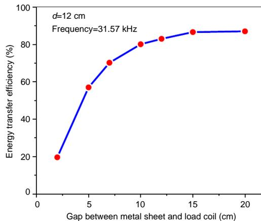
**Figure 8.** The experimental dependence of energy transfer efficiency on the physical spacing between the load coil and the metallic plate.
