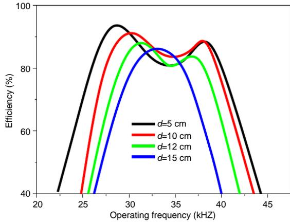
**Figure 3.** Simulated frequency characteristics of energy transfer efficiency for different vertical spacing between the transmitting and receiving resonant coils of wireless energy transfer system.
