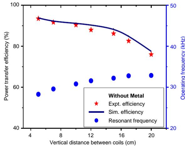
**Figure 5.** Both the simulated and experimental resonant frequency characteristics of optimum energy transfer efficiency of the wireless energy transfer system without metal plate.
