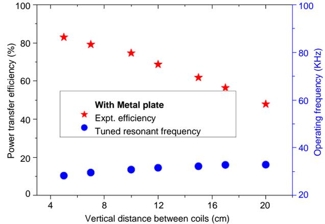
**Figure 7.** Measured frequency characteristics of optimum energy transfer efficiency with different vertical spacing between the coils in the presence of metallic plate.
