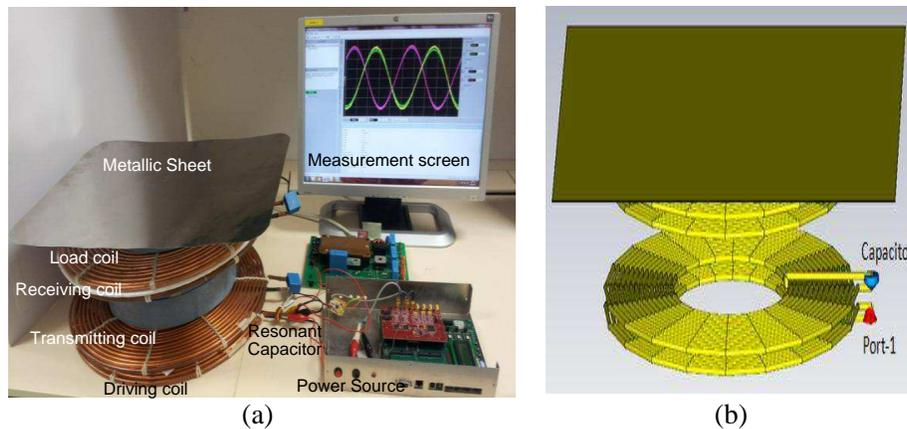
**Figure 2.** Magnetic resonance coupling based wireless energy transfer system with proximal metallic object. (a) Experimental setup. (b) Electromagnetic simulation model.
