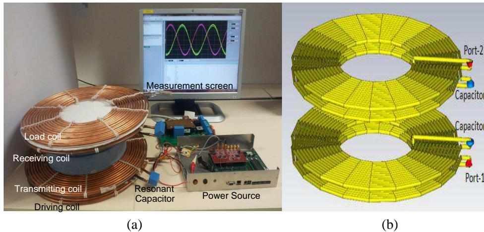
**Figure 1.** Magnetic resonance coupling based wireless energy transfer system for EV charging. (a) Experimental setup. (b) Electromagnetic simulation model.
