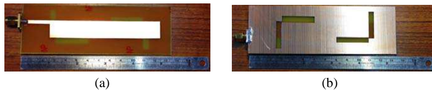
Figure 2. The fabricated proposed antenna. (a) Top layer. (b) Bottom layer.
