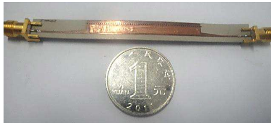
Figure 8. Photograph of the fabricated ferrite-loaded HMSIW phase shifter.
