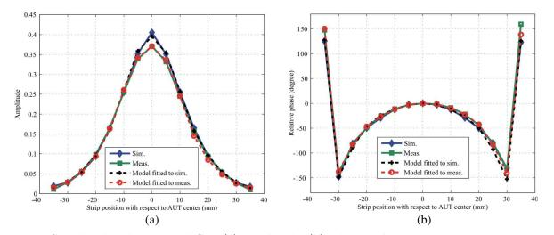
**Figure 5.** Simulated and measured  $S_{11}$ : (a) amplitude; (b) relative phase.
