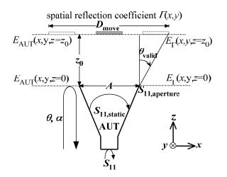
Figure 1. Schematic layout of the proposed antenna pattern retrieval method.
