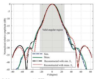
Figure 7. Normalized far-field pattern at 30 GHz.
