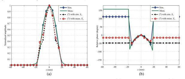
Figure 6. Electric near-field distribution at AUT aperture: (a) normalized amplitude; (b) relative phase.
