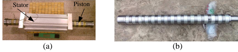
Figure 10. (a) Prototype of PMTLG. (b) Piston of PMTLG.
