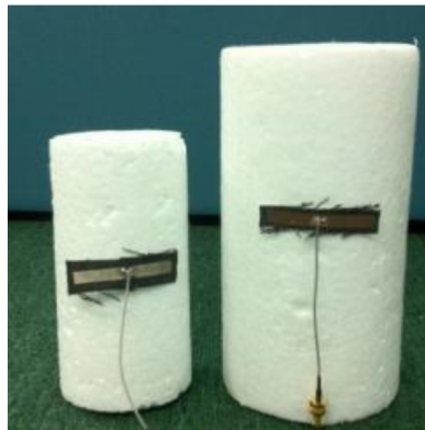
Figure 11. Bending experiments of fully textile dipole antenna.
