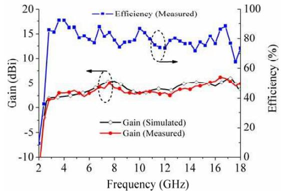
**Figure 7.** Measured and simulated antenna gains and measured radiation efficiency of the proposed dipole antenna.
