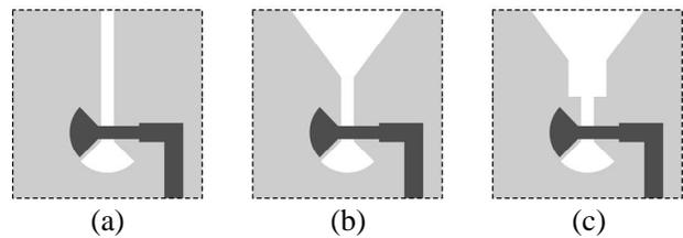
**Figure 3.** Comparisons of the simulated reflection coefficients of the printed dipole antenna with three feeding structures, (a) uniform feeding structure, (b) beveled feeding structure, and (c) proposed beveled offset feeding structure.
