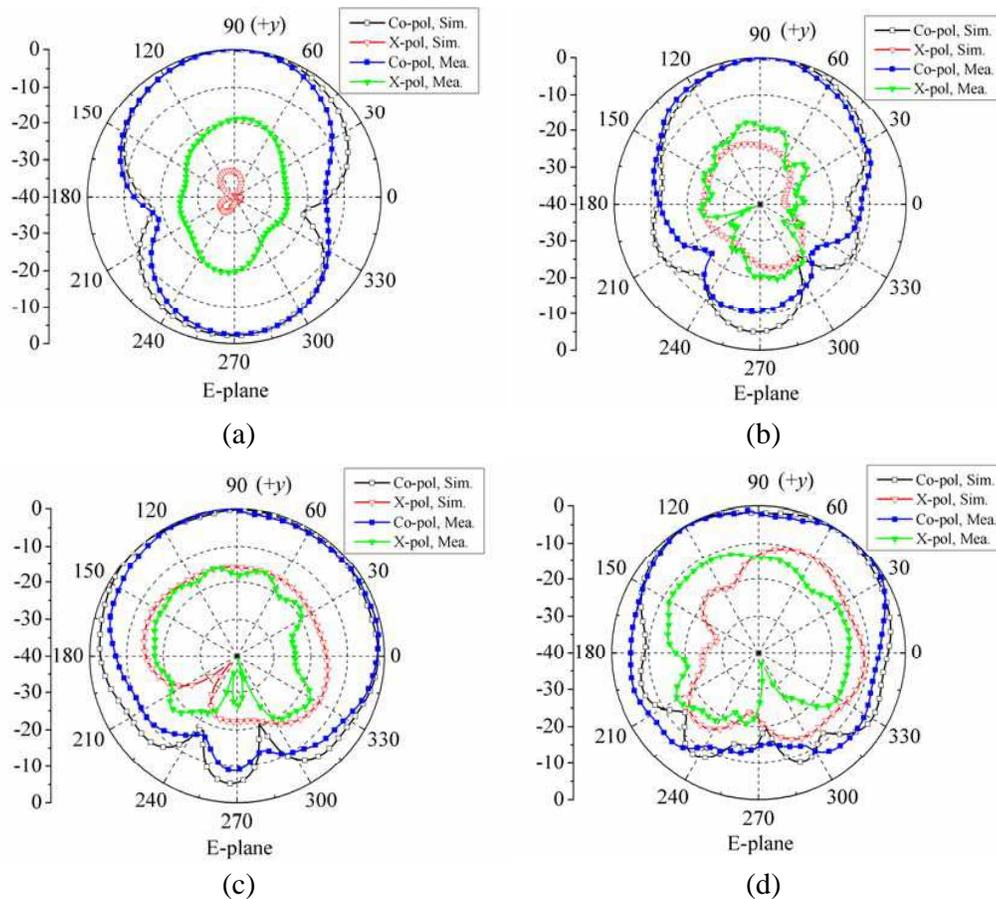
**Figure 8.** Simulated and measured radiation patterns of the proposed antenna in  $E$ -plane ( $xy$ -plane) at the different frequencies, (a) 4 GHz, (b) 8 GHz, (c) 12 GHz, (d) 16 GHz.
