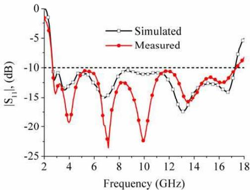
**Figure 6.** Measured and simulated reflection coefficients of the designed dipole antenna.
