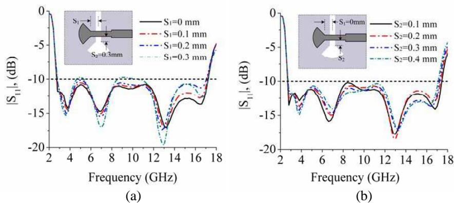
**Figure 4.** Effect of the misalignment between the bottom and the top layers on the reflection coefficients of the designed dipole antenna, (a)  $S_1$ , and (b)  $S_2$ .
