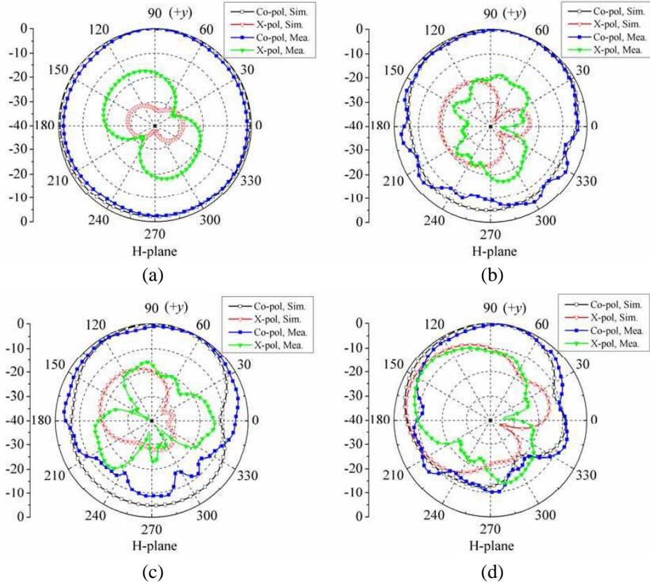
**Figure 9.** Simulated and measured radiation patterns of the proposed antenna in  $H$ -plane ( $yoz$ -plane) at the different frequencies, (a) 4 GHz, (b) 8 GHz, (c) 12 GHz, (d) 16 GHz.
