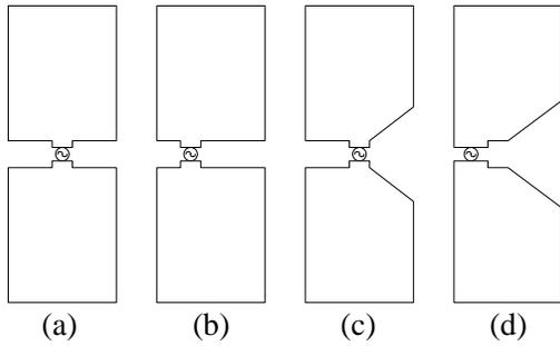
**Figure 1.** The printed dipole antenna with different feeding mechanisms, (a) center-fed, (b) offset-fed, (c) beveled center-fed, and (d) beveled offset-fed.
