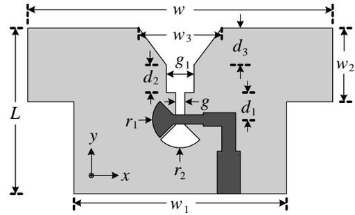
**Figure 2.** Geometry of the proposed printed dipole antenna.
