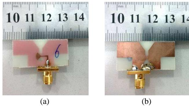
**Figure 5.** Photographs of the fabricated antenna, (a) top layer, (b) bottom layer.
