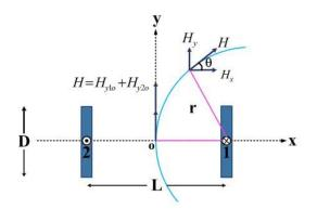
Figure 5. Model of PM by single current sheet.
