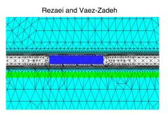
Figure 7. Mesh generation of PEDS model.
