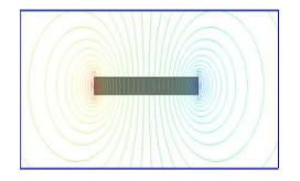
Figure 8. Magnetic flux paths around the PM.
