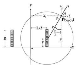
Figure 1. Physical model of electo-dynamic suspension system.
