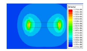
Figure 9. Magnetic field spectrum around the PM.
