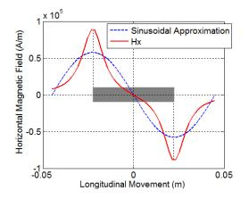
Figure 3. Horizontal magnetic field and its fundamental component.
