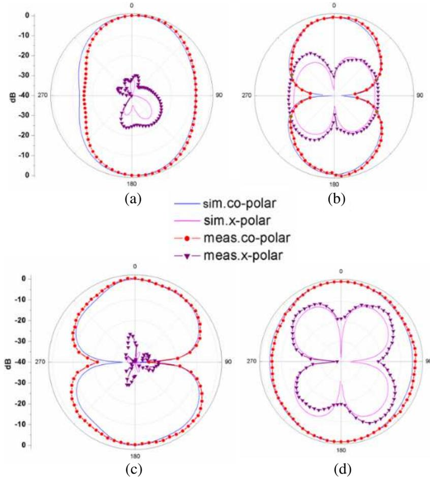
**Figure 9.** Measured and simulated radiation patterns at 2.3 GHz for port 1 (a)  $XZ$ -plane and (b)  $YZ$ -plane and port 2 (c)  $XZ$ -plane and (d)  $YZ$ -plane.
