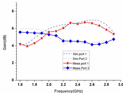
**Figure 11.** Measured and simulated gains for the proposed antenna.
