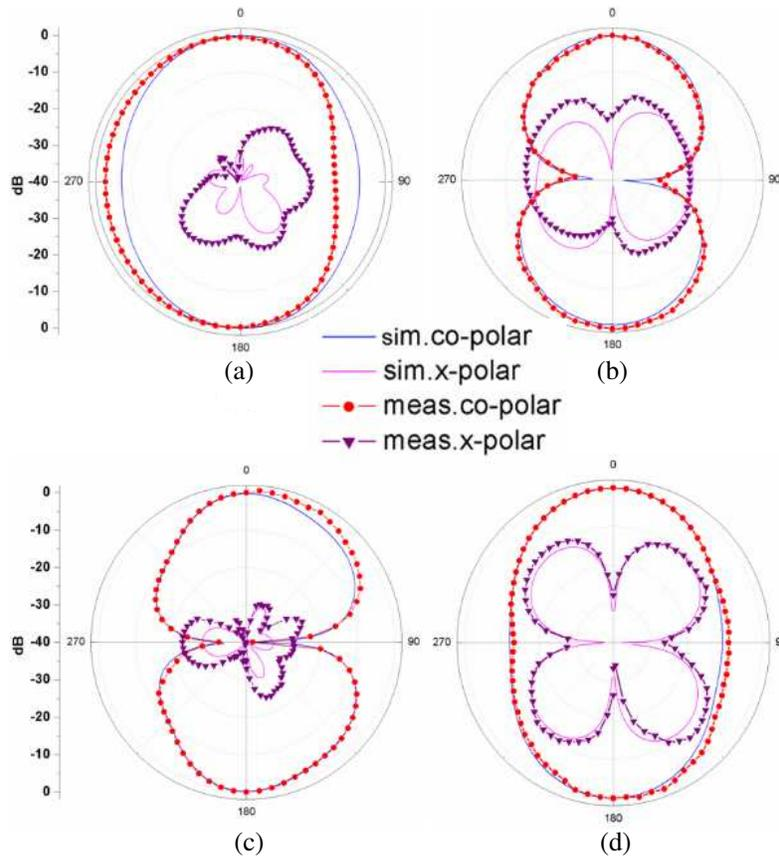
**Figure 8.** Measured and simulated radiation patterns at 1.9 GHz for port 1 (a)  $XZ$ -plane and (b)  $YZ$ -plane and port 2 (c)  $XZ$ -plane and (d)  $YZ$ -plane.
