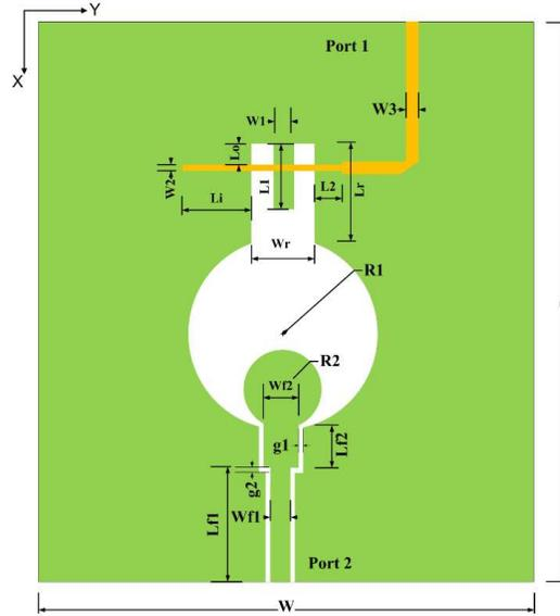
**Figure 1.** Geometry of the proposed antenna. Some of the optimized key parameters are listed as follows:  $L = 175$ ,  $W = 125$ ,  $L_{f1} = 34$ ,  $L_{f2} = 13.8$ ,  $W_{f1} = 3.8$ ,  $W_{f2} = 5.4$ ,  $g_1 = 0.3$ ,  $g_2 = 0.5$ ,  $R_1 = 31$ ,  $R_2 = 12$ ,  $W_1 = 2.4$ ,  $W_r = 5.2$ ,  $W_2 = 1$ ,  $W_3 = 1.5$ ,  $L_1 = 12$ ,  $L_2 = 2$ ,  $L_i = 8.8$ ,  $L_r = 25$ ,  $L_o = 6$  (Units: mm).
