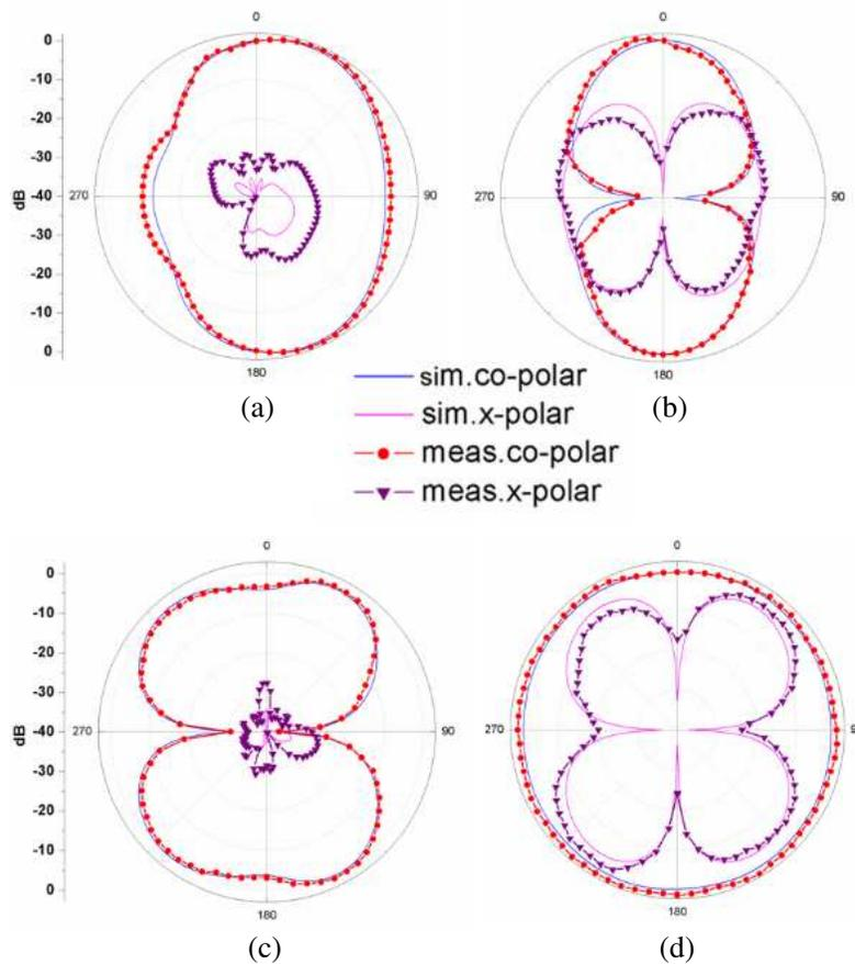
**Figure 10.** Measured and simulated radiation patterns at 2.6 GHz for port 1 (a) XZ-plane and (b) YZ-plane and port 2 (c) XZ-plane and (d) YZ-plane.
