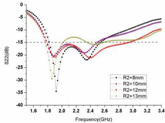
Figure 4. Simulated  $|S_{22}|$  of the proposed antenna with different  $R_2$ .
