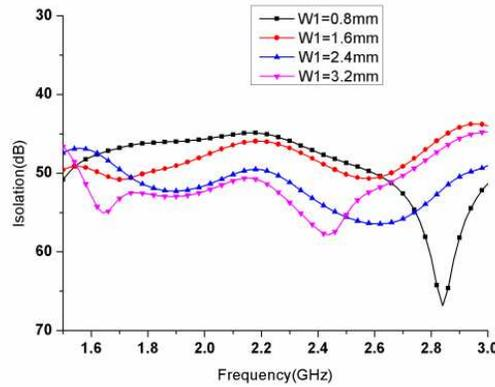
**Figure 5.** Simulated isolation of the proposed antenna with different  $W_1$ .
