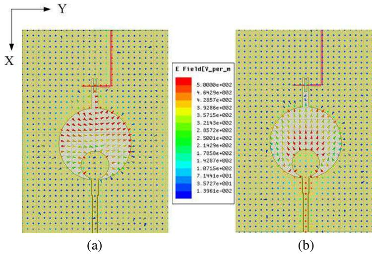
Figure 2. Electric fields in circular slot at 2.3 GHz: fed by (a) Port 1 and (b) Port 2.
