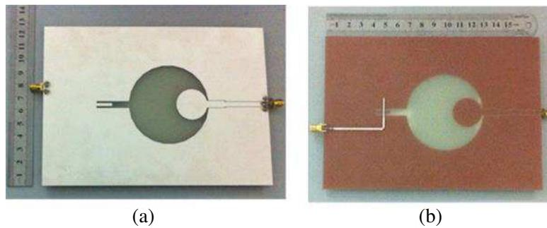
**Figure 6.** Photographs of the proposed antenna (a) top and (b) bottom view.
