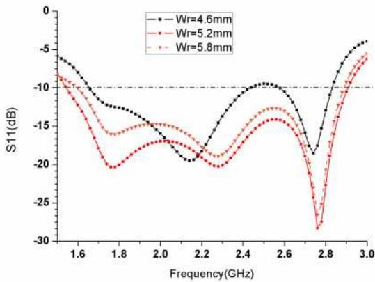
Figure 3. Simulated  $|S_{11}|$  of the proposed antenna with different  $W_r$ .
