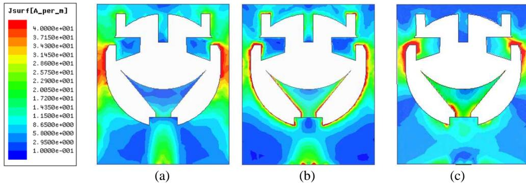
**Figure 3.** Simulated surface current distributions of the proposed antenna at (a) 2.5, (b) 3.5, and (c) 5.5 GHz.
