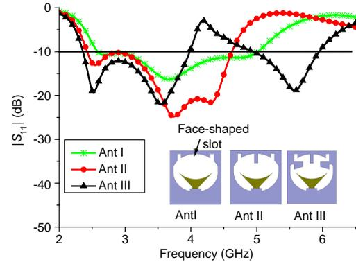
**Figure 2.** Simulated return loss of various antennas.
