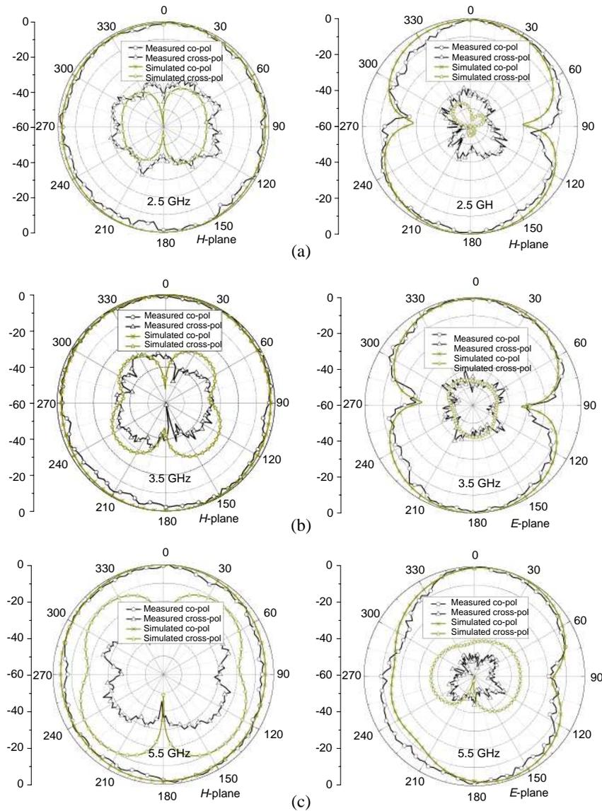
**Figure 7.** Radiation patterns of the proposed antenna at (a) 2.5, (b) 3.5, and (c) 5.5 GHz.
