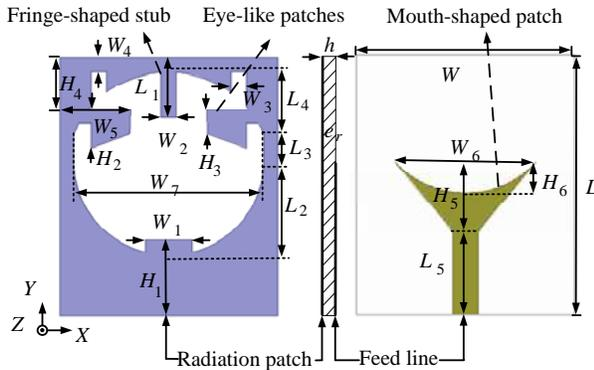
**Figure 1.** Geometry of the antenna.
