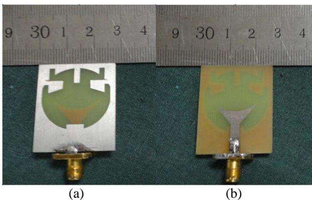
**Figure 5.** Photograph of the fabricated antenna: (a) front view, (b) back view.
