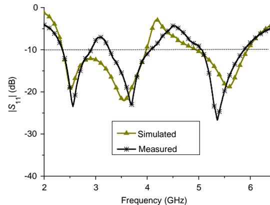
**Figure 6.** Measured and simulated return losses of the proposed antenna.
