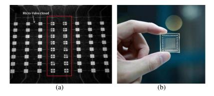
**Figure 5.** (a) Captured CCD image of the microfluidic device. The vertical micro-valves are closed to allow sample flows vertically. The diamond-shaped dark areas in the gold spots are regions where SPR occur. (b) Photograph of the microfluidic chip.
