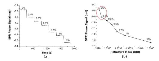
**Figure 6.** (a) Real time recorded SPR signal when the probe channel is injected with different glycerine solutions. (b) The mean values and the standard deviations of the SPR phase signal with different refractive index solutions.
