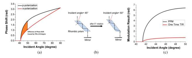
**Figure 1.** (a) Curves of the simulated phase shifts of p- and s-polarization light for one time total internal reflection. The glass refractive index is set to be 1.515 in the simulation. (b) The arrangement of PPM (the rotation stage is not shown) and the detailed light-path in therhombic prism when the incident angle is 45 degree (left) and 50 degree (right), respectively. (c) The modulation result for one time TIR and the PPM (8 times TIR).
