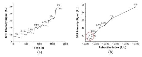
**Figure 7.** (a) Intensity signal of p-polarization light when the probe channel is injected with different glycerine solutions. (b) The mean values and the standard deviations of the SPR intensity signal with different refractive index solutions.
