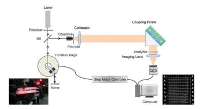
**Figure 2.** Schematic diagram the setup of our PPM-based SPR sensor. BS stands for beam splitter. The left-bottom inset is the photograph of the PPM. The right-bottom inset shows the SPR image of a homemade microfluidic channels captured by the CCD.
