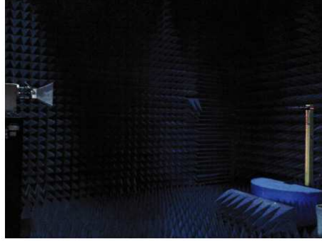
Figure 15. The measurement setup in anechoic chamber.
