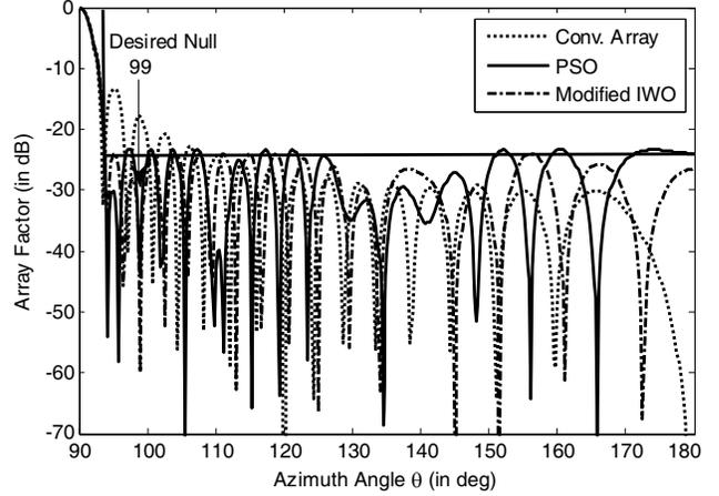
**Figure 8.** The normalized array pattern of 32-element linear array obtained by modified IWO with constraint handling, with desired null at  $99^\circ$ .
