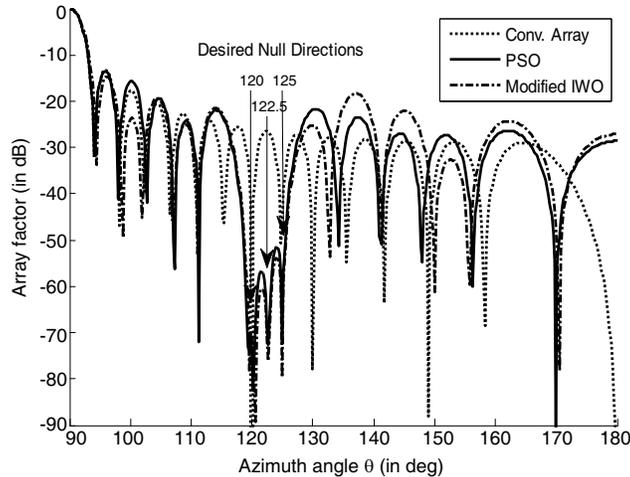
**Figure 4.** The normalized array pattern of 28-element linear array optimized using modified IWO with desired nulls at  $120^\circ$ ,  $122.5^\circ$  and  $125^\circ$ .
