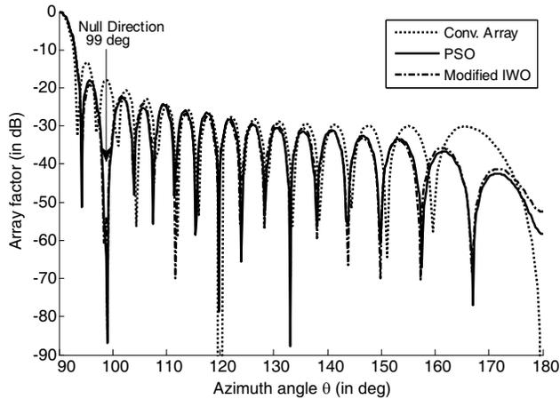
**Figure 5.** The normalized array pattern of 32-element linear array obtained by modified IWO with desired null at 99°.
