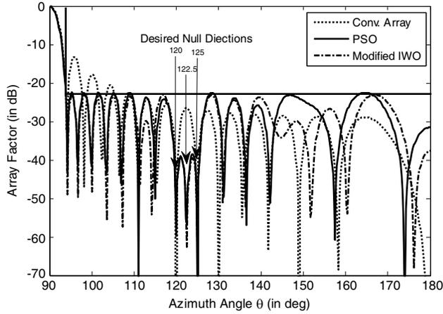
**Figure 7.** The normalized array pattern of 28-element linear array obtained by modified IWO with constraint handling, with desired nulls at  $120^\circ$ ,  $122.5^\circ$  and  $125^\circ$ .
