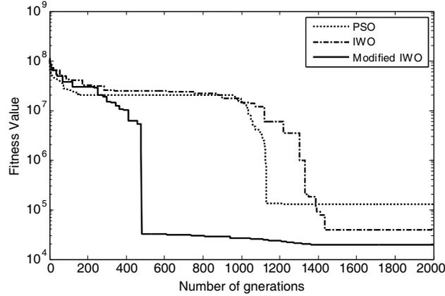
**Figure 9.** The convergence characteristics of the PSO, IWO and modified IWO with constraint handling for a 32 element linear array.
