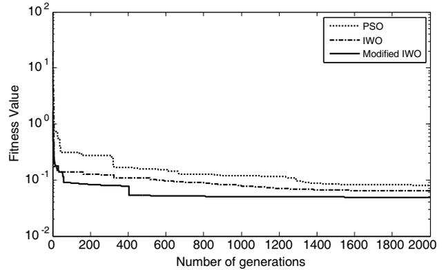
**Figure 6.** The convergence characteristics of the PSO, IWO and modified IWO algorithms for optimization of a 32 element linear array.
