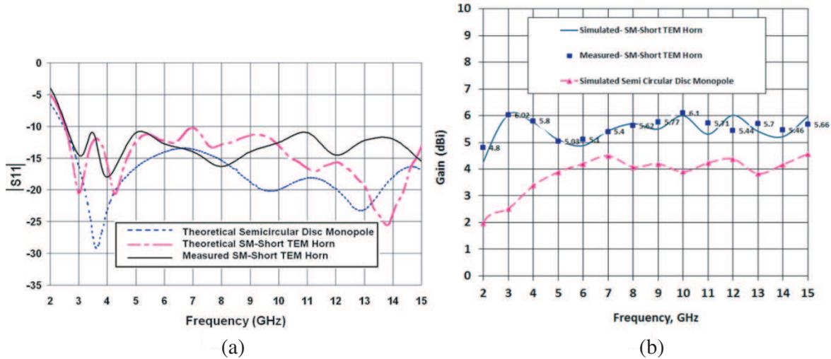
**Figure 4.**  $|S_{11}|$  of the CPW-fed disc monopole antenna with and without the short horn. (b) Comparison of the measured peak gain of the CPW-fed disc monopole antenna, with and without the short horn.
