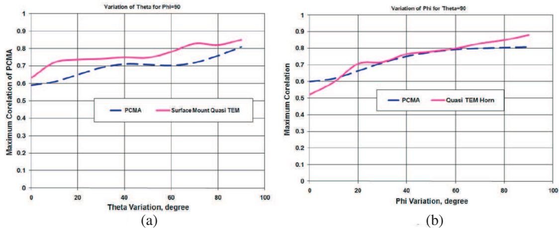
Figure 6. Pulse correlation of the new antenna and the reference semicircular disc monopole antenna, where theta is varying from Y to Z in yz-plane and phi is variation from X to Z in xz-plane.
