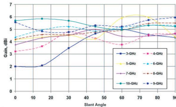
Figure 3. Simulated gain vs. slant angle ( $\alpha$ ), in degrees, for different frequencies.
