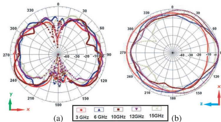
**Figure 5.** Measured radiation patterns. (a) X-Y plane. (b) X-Z plane.
