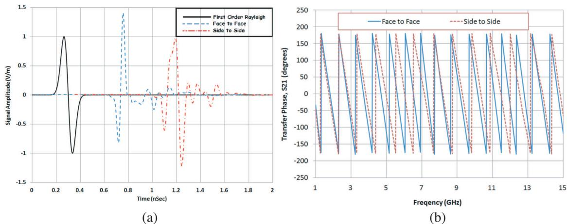
Figure 7. (a) Pulse performance of antenna. (b) Transmission phase of the new antenna for face to face and side to side arrangements.
