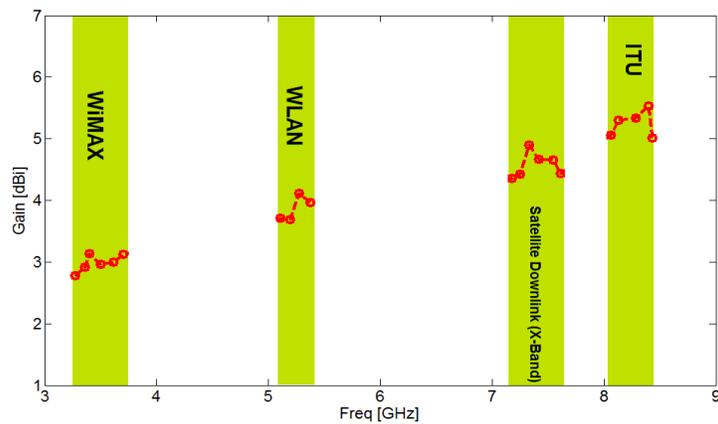
Figure 10. Measured maximum gain of the proposed antenna.
