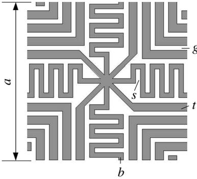
**Figure 1.** UC-EBG structure cell.
