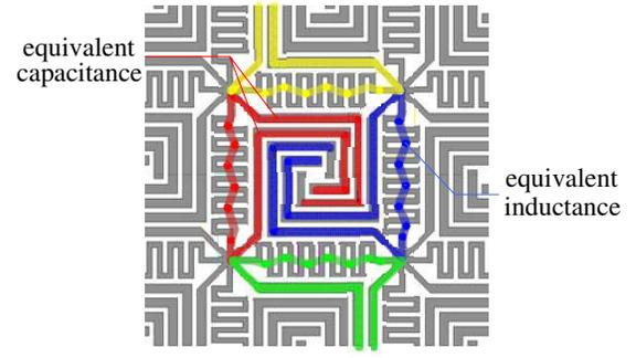
**Figure 2.** UC-EBG structure and its equivalent  $LC$  circuit.
