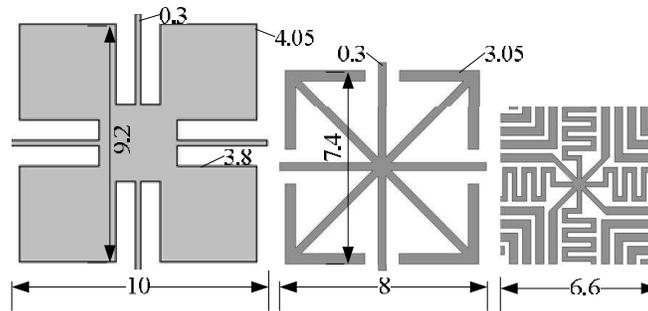
**Figure 5.** Size comparison of UC-EBG structure (unit: mm).
