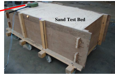
Figure 12. Sand test bed used for scattering experiment.
