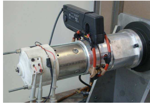
Figure 16. Prototype with slip rings for internal measurements.
