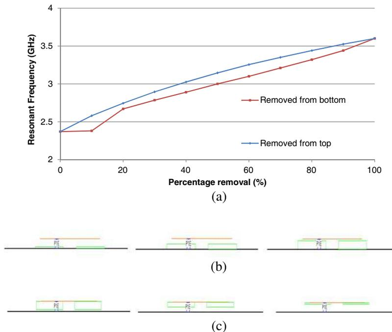
**Figure 8.** Simulated results with variation in substrate height. (a) Removing substrate from top and bottom; (b) substrate removed from top and (c) substrate removed from bottom.
