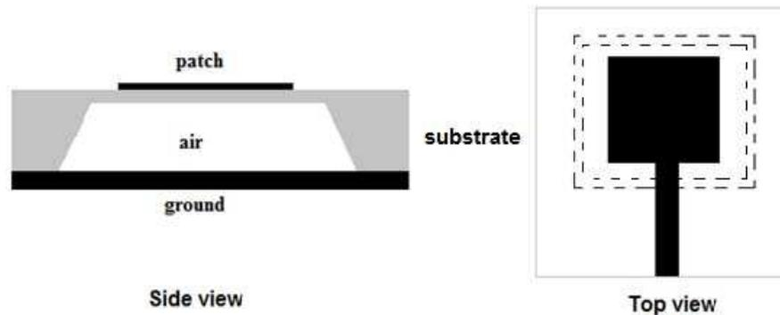
**Figure 2.** A micromachined patch antenna. The dotted boundary in the top marks the start and the end of the slanted edges. The edges are slanted due to anisotropic chemical etching (redrawn from [13]).
