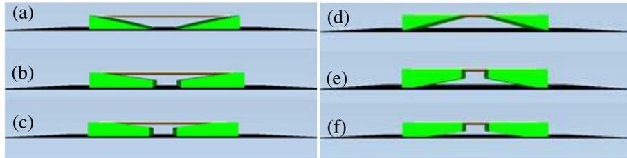
**Figure 9.** Triangular sections of substrate removed: (a)–(c) from top; (d)–(f) from bottom.
