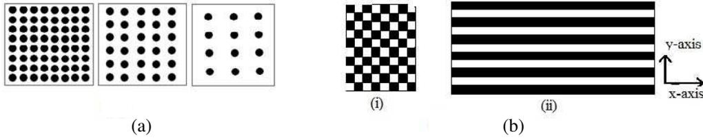
**Figure 3.** (a) A perforated dielectric slab where the density of air-filled holes varies the effective permittivity (redrawn from [26]); (b) the darker part indicates the section from which the substrate has been removed. The direction of electric field is along  $z$ -axis for (i) and  $y$ -axis for (ii) (redrawn from [27]).
