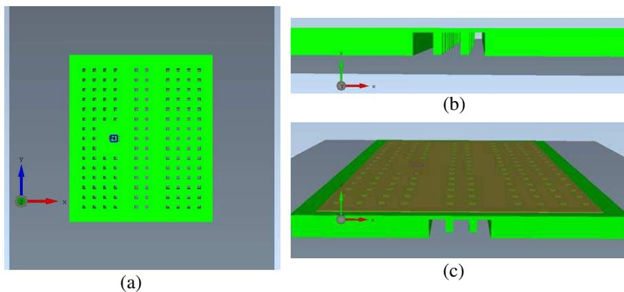
**Figure 10.** Geometry of final design. (a) Top view of final design of substrate with holes; (b) side view showing legs supporting the central structure and (c) including patch (the patch is continuous but is transparent to show the holes in the substrate).
