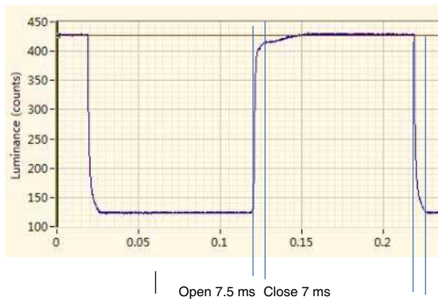
Figure 9. Switching response time of electrofluidic display pixels.
