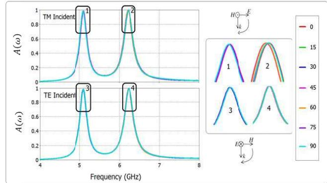
**Figure 12.** Simulated angular dependency of the absorption properties for *TE* and *TM* waves.
