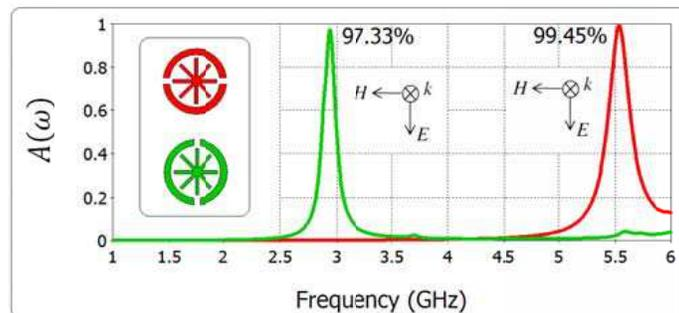
**Figure 5.** Simulated absorptivity of the modified MA.
