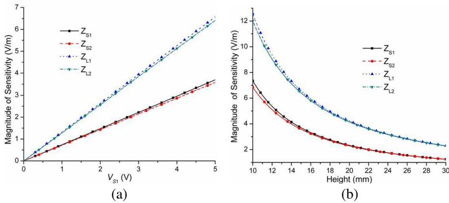
Figure 5. The sensitivities of the load voltages change with the terminal voltage  $V_{S1}$  and the height of the transmission line. (a) Changing with the terminal voltage. (b) Changing with the height.
