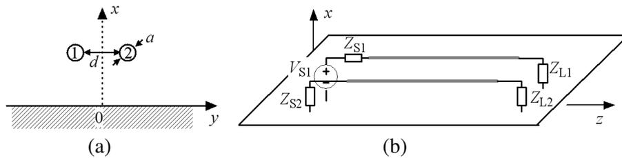
**Figure 2.** The model to be analyzed. (a) Cross section. (b) Configuration.
