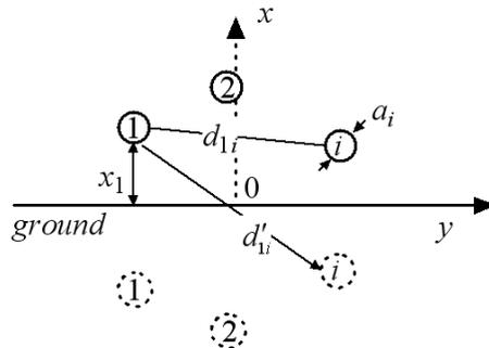
**Figure 1.** A multiconductor transmission line over the ground.
