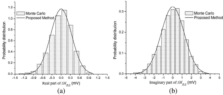
Figure 4. The probability distribution of  $\Delta V_{ZL2}$ . (a) The real part. (b) The imaginary part.
