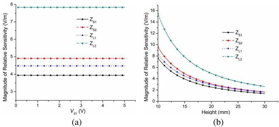
Figure 6. The relative sensitivities of the load voltages change with the terminal voltage  $V_{S1}$  and the height of the transmission line. (a) Changing with the terminal voltage. (b) Changing with the height.
