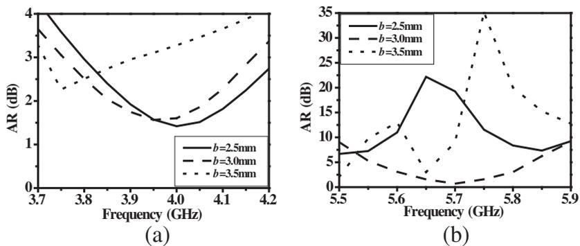
Figure 12. Simulated AR with different slit height.
