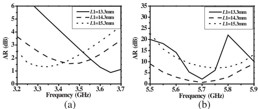
Figure 10. Simulated AR with different square loop size.
