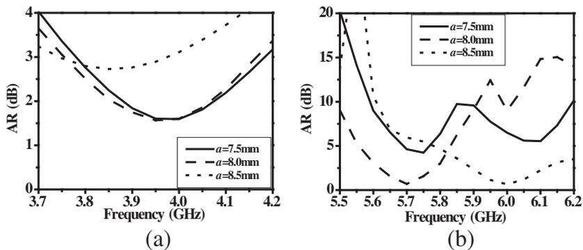
Figure 11. Simulated AR with different slit length.
