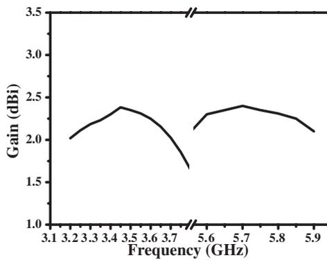
**Figure 9.** Measured gain of the proposed antenna.
