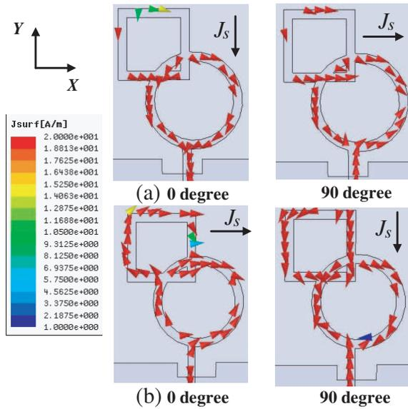
**Figure 2.** Simulated current distributions: (a) 3.52 GHz and (b) 5.75 GHz.
