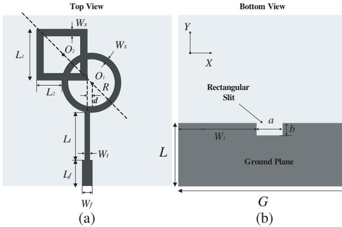
**Figure 1.** Configurations of the proposed antenna. (a) Top view; (b) Bottom view.
