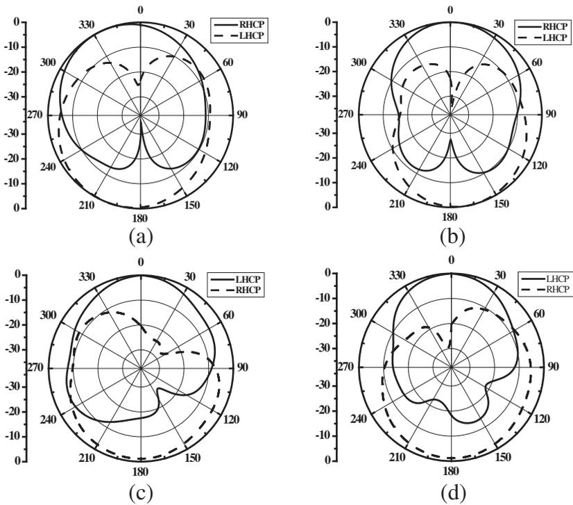
**Figure 8.** Measured radiation patterns of the proposed dual-band CP antenna. (a) 3.5 GHz at  $\varphi = 0^\circ$ ; (b) 3.5 GHz at  $\varphi = 90^\circ$ ; (c) 5.75 GHz at  $\varphi = 0^\circ$ ; (d) 5.75 GHz at  $\varphi = 90^\circ$ .
