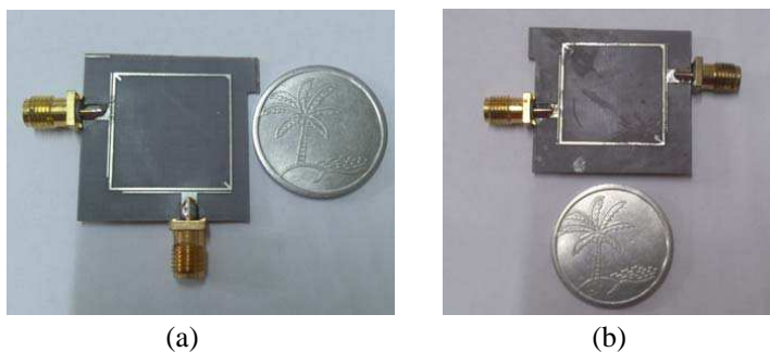
Figure 9. Fabricated photographs of (a) Filter I, the dimensions are: L = 21.6 , L_1 = 1.16 , L_2 = 10.6 , L_3 = 6.3 , W = 0.5 , W_1 = 0.5 , W_2 = 0.3 , W_3 = 2.73 , p = 0.71 , and (b) filter II, the dimensions are: L = 21.2 , L_1 = 0.88 , L_2 = 9.1 , L_3 = 5.1 , W = 0.5 , W_1 = 0.5 , W_2 = 0.3 , W_3 = 2.73 , p = 0.71 , D = 1 (in mm).
