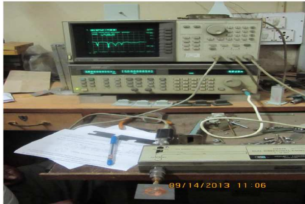
Figure 7. Measurement of return loss of CFA using network analyzer.
