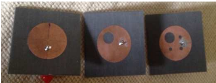
Figure 5. Fabricated structures for 0th, 1st and 2nd iteration of CFA.
