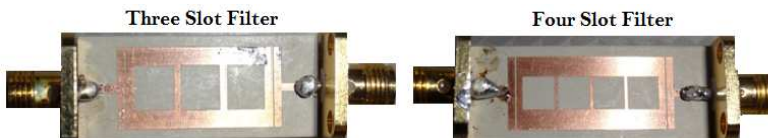
Figure 14. Photograph of the fabricated prototypes of the 3-slot and 4-slot multiband band pass filters.
