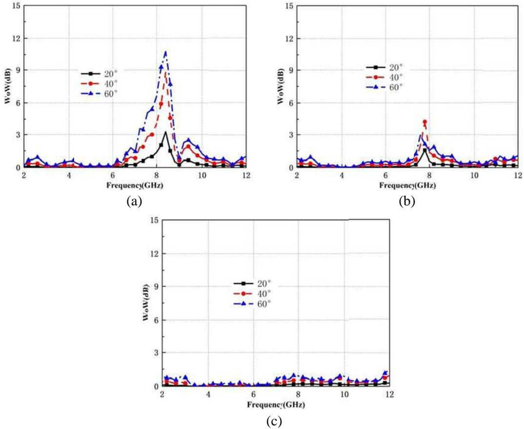
**Figure 10.** WoW of the improved antenna versus frequency with different center section radii. (a)  $R = 7$  mm. (b)  $R = 10$  mm. (c)  $R = 13$  mm.
