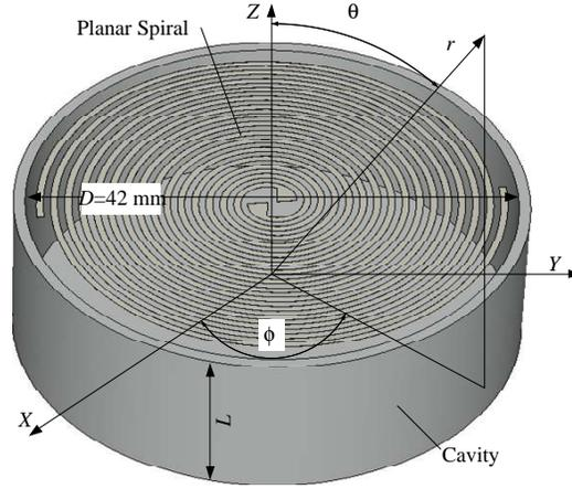
**Figure 1.** Configuration of cavity backed planar spiral antenna.
