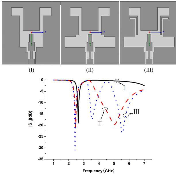
**Figure 2.** Configuration of the three antennas and simulated results against frequency for the proposed antenna with/without second slot, third slot loading.
