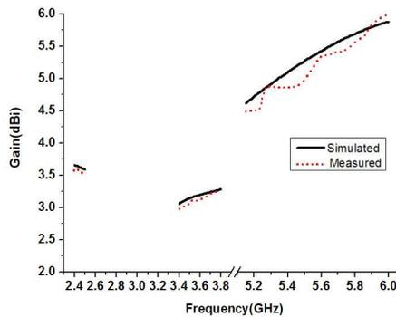
**Figure 8.** Simulated and measured gains of the proposed antenna for frequencies across the 2.4–2.5 GHz, 3.4–3.8 GHz and 5.15–6.0 GHz bands.
