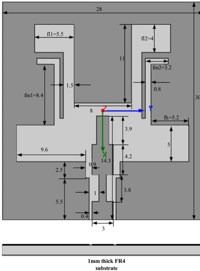
**Figure 1.** Schematic configurations of proposed CPW-fed antenna (unit: mm).
