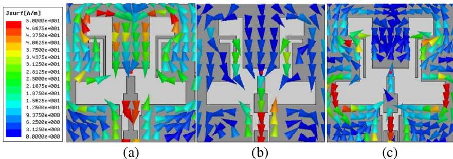
**Figure 3.** Simulated results of the surface current distributions for the proposed triple-frequency slot antenna studied in Figure 2 at (a) 2.4 GHz, (b) 3.6 GHz, (c) 5.5 GHz.
