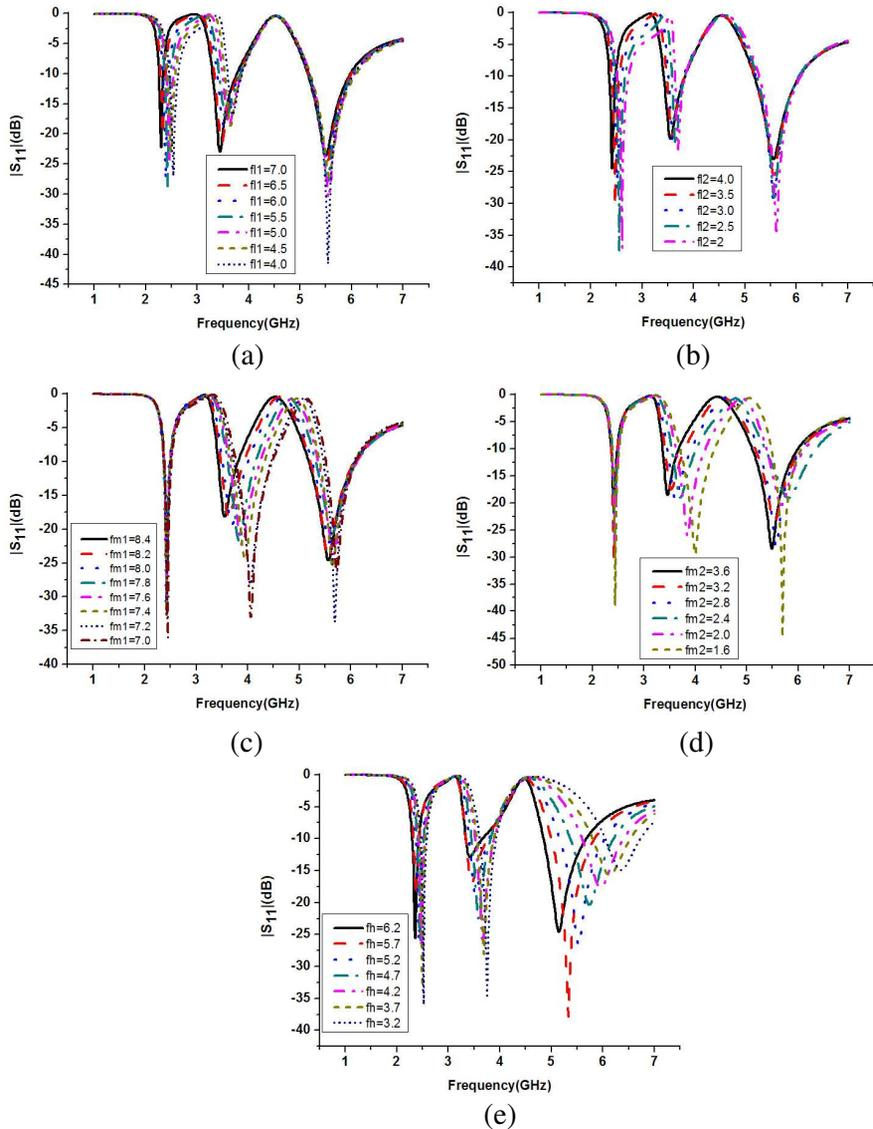
**Figure 4.** Simulated return loss against frequency for the proposed triple-frequency slot antenna with various (a)  $f_{l1}$ , (b)  $f_{l2}$ , (c)  $f_{m1}$ , (d)  $f_{m2}$  and (e)  $f_h$ , other parameters are the same as shown in Figure 1.
