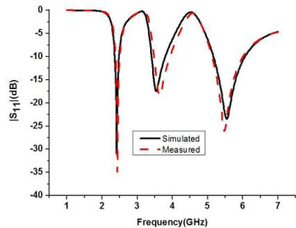
**Figure 6.** Measured and simulated return loss against frequency for the proposed CPW-fed slot antenna.
