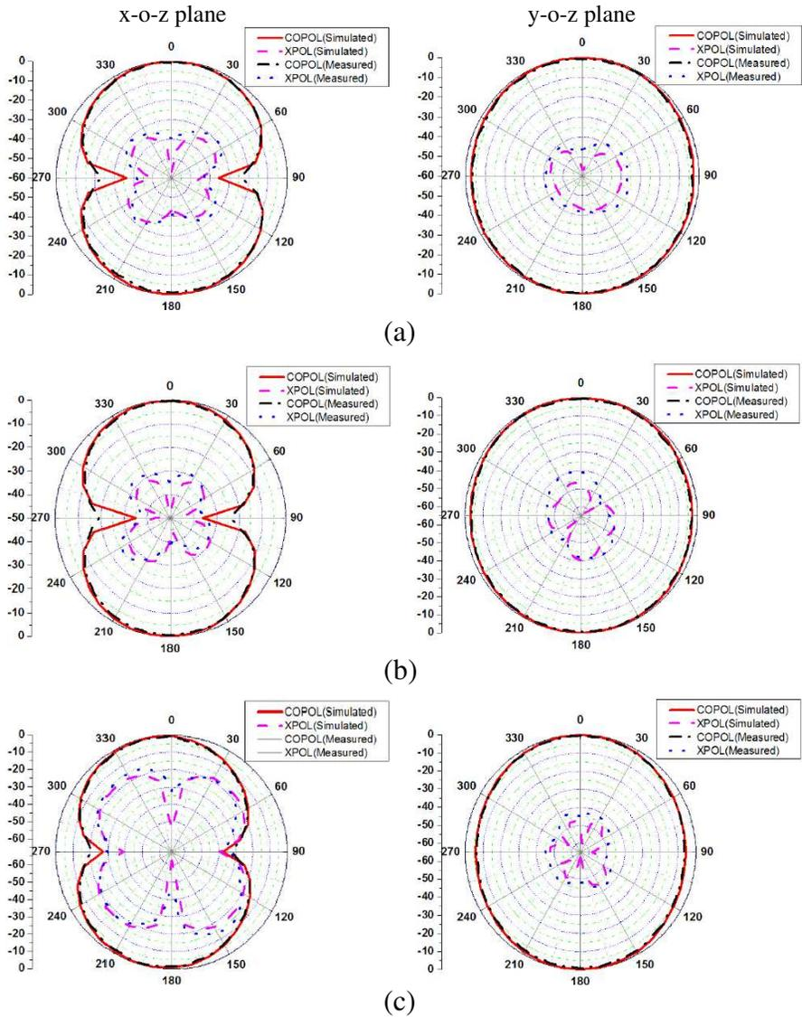
**Figure 7.** Simulated and measured radiation patterns of the proposed triple-frequency antenna at (a) 2.4 GHz, (b) 3.6 GHz, and (c) 5.5 GHz. *E*-plane (*x-z* plane), *H*-plane (*y-z* plane).
