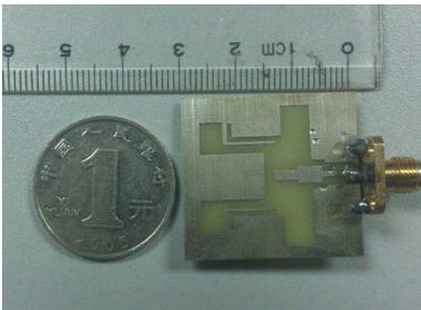
**Figure 5.** Fabricated dual-band antenna.
