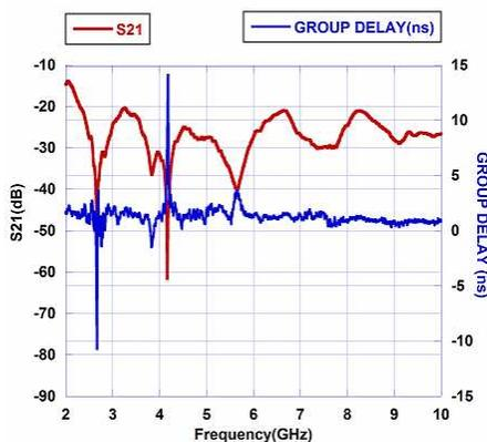
**Figure 10.** Measured group delay and transfer function of the proposed band notched UWB antenna.
