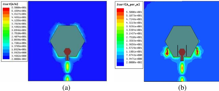
**Figure 5.** Surface current distributions of the (a) reference and (b) proposed structure at 3.8 GHz.
