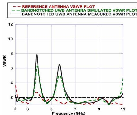
**Figure 3.** Comparison between simulated and measured VSWR responses of proposed band notched UWB antenna and reference UWB antenna.
