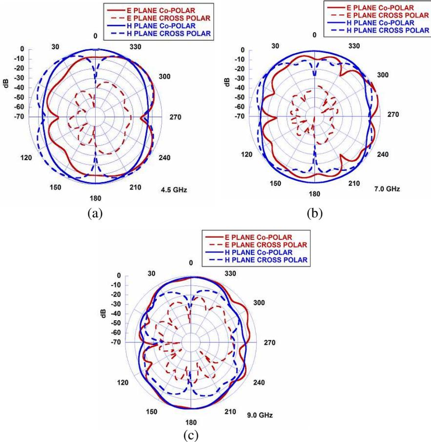
**Figure 7.** *E*-plane and *H*-plane radiation patterns at (a) 4.5 GHz, (b) 7.0 GHz, (c) 9.0 GHz.
