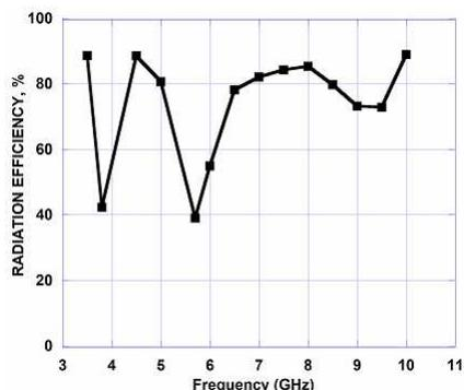
**Figure 9.** Simulated radiation efficiency versus frequency for band-notched UWB antenna.
