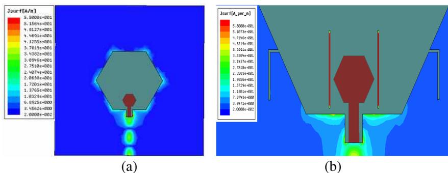
**Figure 6.** Surface current distributions of the (a) reference and (b) proposed structure at 5.7 GHz.
