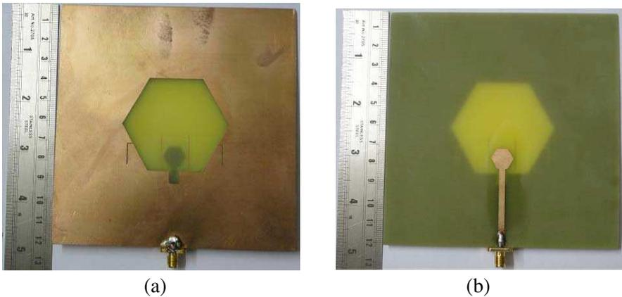
**Figure 2.** (a) Slot-side view of the prototype. (b) Feed-side view of the prototype.
