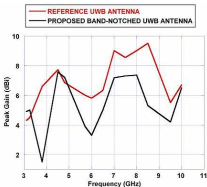
**Figure 8.** Simulated peak antenna gain versus frequency for band-notched UWB antenna and reference UWB antenna.
