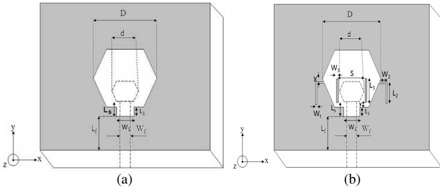
**Figure 1.** Schematic diagram of (a) reference UWB antenna. (b) Proposed band-notched UWB antenna.
