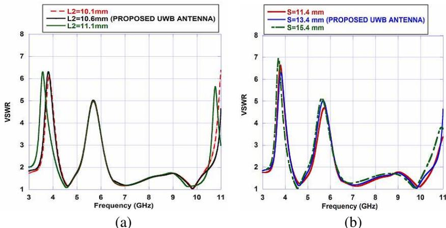
**Figure 4.** (a) Simulated VSWR response of proposed antenna for different values of  $L_2$ . (b) Simulated VSWR response of proposed antenna for different values of  $S$ .
