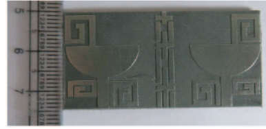
Figure 17. Fabricated antenna with cross-strip VFSS.
