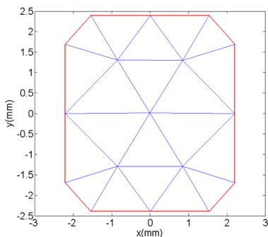
**Figure 5.** Geometries and meshing of the iris.
