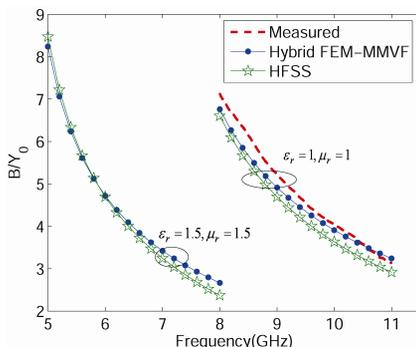
Figure 3. Relative susceptance of the cross-shaped iris.
