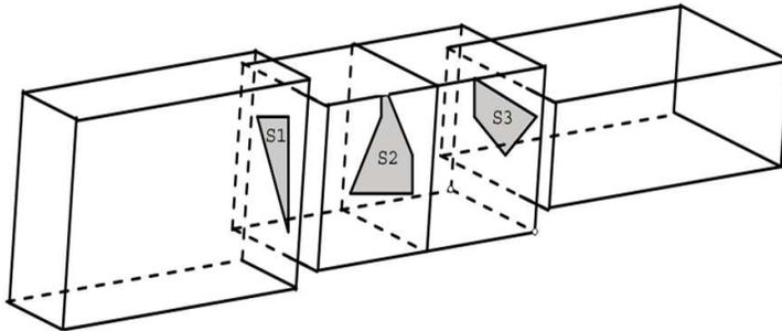
**Figure 1.** Waveguide filter with cascaded complex discontinuities.
