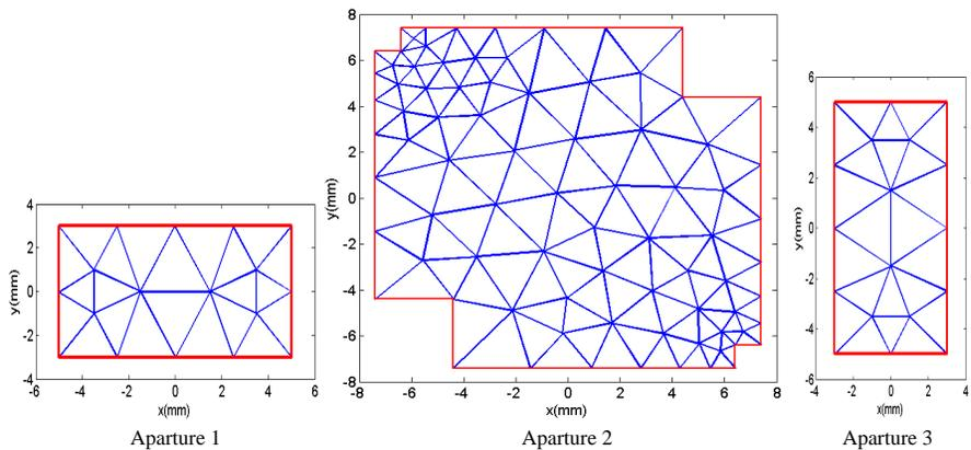
Figure 10. Geometries and meshing the three apertures.
