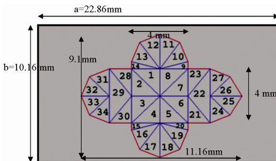
Figure 2. Geometries and meshing of the cross-shaped aperture.
