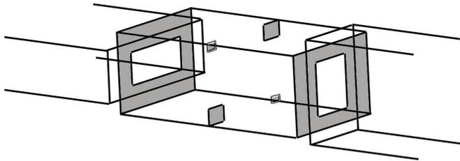
Figure 9. Dual-mode filter.
