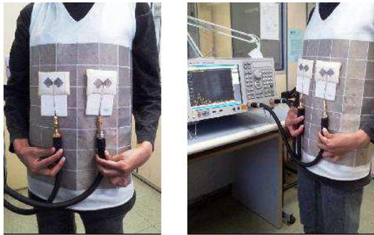
**Figure 16.** Textile AMC jacket on-body measurement.
