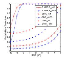
Figure 1. Probability of detection versus SNR for different probability of false alarm with N = 256 and M = 8.
