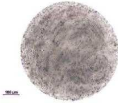
Figure 8. Photograph of Ca-alg microsphere homogeneously loaded with iron particles.
