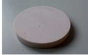
Figure 2. Fabricated sample of W19 epoxy and Ca-alg spheres as inclusions.
