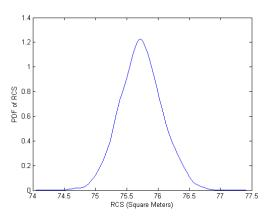
Figure 6. Probability density function for the radar cross section of an array of cylindrical conductors for Benchmark Problem 4.
