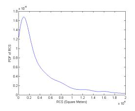
Figure 7. Probability density function for the radar cross section of an array of cylindrical conductors for Benchmark Problem 5.
