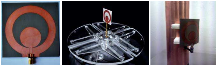
Figure 9. Photographs of the fabricated antenna and antenna placed on a tower in anechoic chamber.
