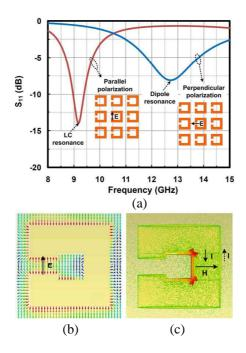
**Figure 4.** (a) Simulated response of C-shaped metamaterial absorber for the parallel and perpendicular polarizations, (b) induced electric field, and (c) induced surface current due to magnetic field.
