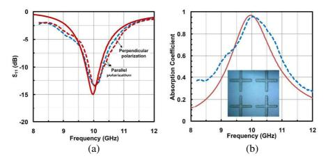
**Figure 9.** Measured (dashed lines) and simulated (continuous lines) results of cross dipole metamaterial absorber, (a) *S*-parameters and (b) absorption coefficients.
