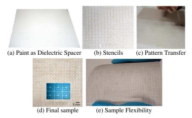
Figure 3. Optical photographs of the sample at different stages during the metamaterial absorber fabrication using paint process. (a) Dielectric paint spacer (1 mm thick) with back side metal layer, (b) metamaterial patterned stencils on paper prepared by laser cutting machine, (c) process of metamaterial pattern transfer on paint spacer layer through stencils, (d) metamaterial patterns on sample after stencil is peeled off, and (e) showing flexibility of samples made.
