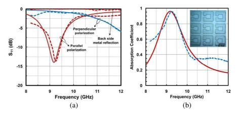
**Figure 7.** Measured (dashed lines) and simulated (continuous lines) results of C-shaped metamaterial absorber, (a) *S*-parameters and (b) absorption coefficients, inset showing microphotograph of the sample.
