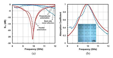
**Figure 8.** Measured (dashed lines) and simulated (continuous lines) results of C-shaped dual-SRR metamaterial absorber, (a) *S*-parameters and (b) absorption coefficients.
