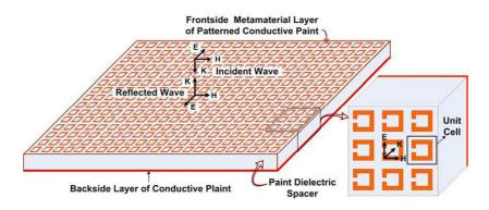
**Figure 1.** Conceptual planar metamaterial absorber: the incident electromagnetic wave is absorbed at metamaterial resonance frequency and reflected back at other frequencies. There is no transmitted wave due to backside metal layer.
