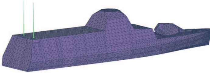
Figure 17. The meshed ship model with two corner HF antennas.
