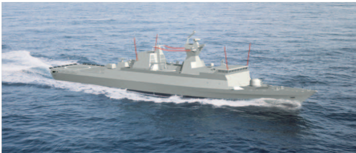
Figure 1. Typical Patrol Vessel (78m of length) and theirs HF antennas in red.
