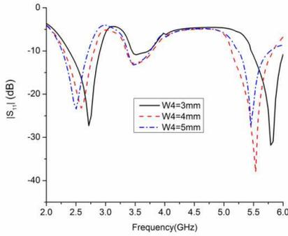
**Figure 10.**  $|S_{11}|$  for different iterations of  $W_4$ .
