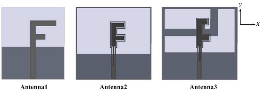
**Figure 3.** Three improved cases of the antenna.
