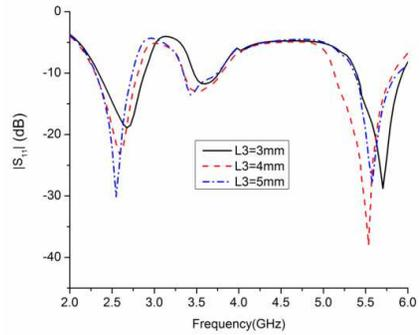
**Figure 9.**  $|S_{11}|$  for different iterations of  $L_3$ .
