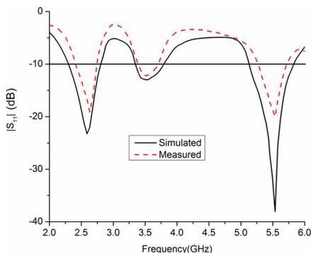
**Figure 6.** Simulated and measured  $|S_{11}|$  variations of the proposed antenna.
