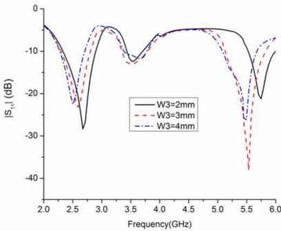
**Figure 8.**  $|S_{11}|$  for different iterations of  $W_3$ .
