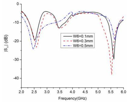
**Figure 11.**  $|S_{11}|$  for different iterations of  $W_6$ .
