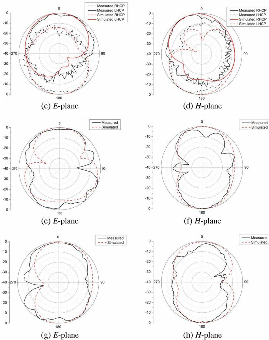
**Figure 14.** The *E*- and *H*-plane radiation pattern of the proposed tri-band antenna at (a)–(b) 2.4 GHz, (c)–(d) 3.5 GHz, (e)–(f) 5.2 GHz, (g)–(h) 5.8 GHz.
