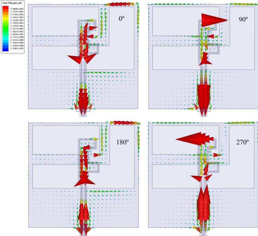
**Figure 7.** Distribution of the surface current on the feed and ground of the proposed antenna at 3.5 GHz in 0°, 90°, 180°, and 270° phase.
