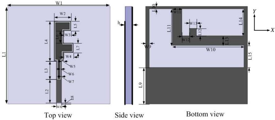
**Figure 1.** Geometry of the proposed tri-band CP antenna ( $L_1 = 40$ ,  $L_2 = 9.5$ ,  $L_3 = 7.5$ ,  $L_4 = 16.5$ ,  $L_5 = 4$ ,  $L_6 = 5$ ,  $L_7 = 4$ ,  $L_8 = 0.5$ ,  $L_9 = 15$ ,  $L_{10} = 1$ ,  $L_{11} = 15$ ,  $L_{12} = 3$ ,  $L_{13} = 4$ ,  $L_{14} = 11$ ,  $L_{15} = 9$ ,  $W_1 = 42$ ,  $W_2 = 7$ ,  $W_3 = 3$ ,  $W_4 = 4$ ,  $W_5 = 0.8$ ,  $W_6 = 0.3$ ,  $W_7 = 0.3$ ,  $W_8 = 2.4$ ,  $W_9 = 1.5$ ,  $W_{10} = 29.5$ ,  $W_{11} = 4$ ,  $W_{12} = 3$ ,  $W_{13} = 3$ ) (Unit: mm).
