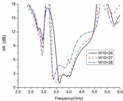
**Figure 12.** AR for different iterations of  $W_{10}$ .
