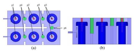
**Figure 8.** The model of six-pole Chebyshev filter. (a) Top view, (b) side view.
