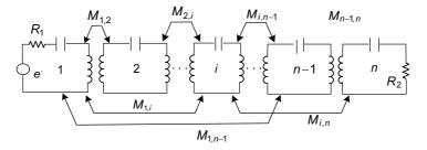
Figure 1. General two-port cross-coupled network.
