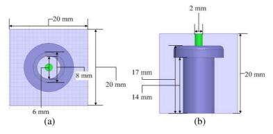
**Figure 4.** The size of single resonator. (a) Bottom view, (b) side view.
