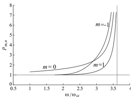
**Figure 3.** Dispersion curves of eigenmodes with the indices  $m = 0, \pm 1$  and  $n = 1$  for  $N = 10^{11} \text{ cm}^{-3}$ ,  $B_0 = 200 \text{ G}$ ,  $\varepsilon_a = 1$ , and  $a = 2.5 \text{ cm}$ .
