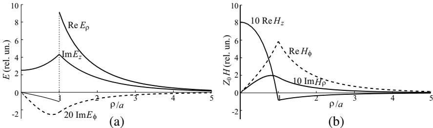
**Figure 4.** Fields (a)  $\mathbf{E}_{m,n}(\rho)$  and (b)  $\mathbf{H}_{m,n}(\rho)$  of an eigenmode with the indices  $m = 0$  and  $n = 1$  for  $N = 10^{11} \text{ cm}^{-3}$ ,  $B_0 = 200 \text{ G}$ ,  $\varepsilon_a = 1$ ,  $a = 2.5 \text{ cm}$ , and  $\omega = 6.6 \times 10^9 \text{ s}^{-1}$ .
