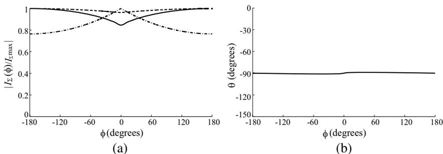
**Figure 5.** Normalized amplitude (a) and phase (b) of the antenna current as functions of the angle  $\phi$  if the antenna is located on the surface of a plasma column (solid line), in free space (dashed line), and in a homogeneous magnetoplasma (dashed-dotted line) for  $a = 0.4$  cm,  $d/a = 0.02$ ,  $\Delta = 0.05$  rad,  $\phi_0 = 0$ ,  $N = 10^{11}$  cm $^{-3}$ ,  $B_0 = 200$  G, and  $\omega = 6.6 \times 10^9$  s $^{-1}$ .
