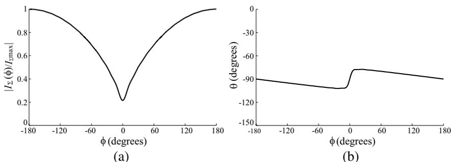
**Figure 6.** Normalized amplitude (a) and phase (b) of the antenna current as functions of the angle  $\phi$  for  $a = 1$  cm,  $d/a = 0.02$ ,  $\Delta = 0.05$  rad,  $\phi_0 = 0$ ,  $N = 10^{11}$  cm $^{-3}$ ,  $B_0 = 200$  G, and  $\omega = 6.6 \times 10^9$  s $^{-1}$ .
