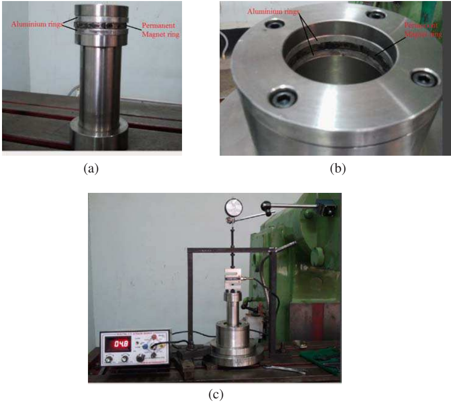
Figure 9. Details of test rig for the measurement of axial force. (a) Arrangement of rings on the inner ring holder (rotor). (b) Arrangement of rings on the outer ring holder (stator). (c) Test rig with load cell and dial gauge.
