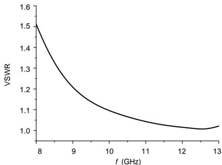
Figure 9. The VSWR of the corrugated-conical horn antenna.
