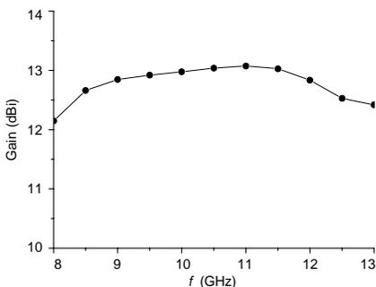
Figure 10. The simulated gain of the corrugated-conical horn antenna.
