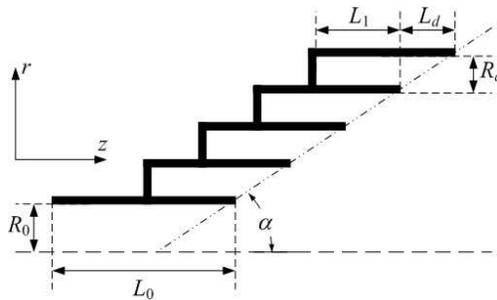
**Figure 7.** Geometry of the corrugated-conical horn antenna.
